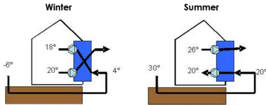
Figure 22 Energy Recovery ventilation (www.concept-bio.eu)
