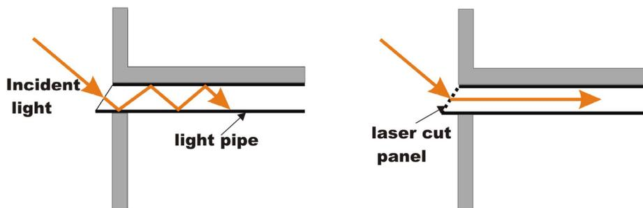
Figure 24 Left: Light pipe with clear glazing.
