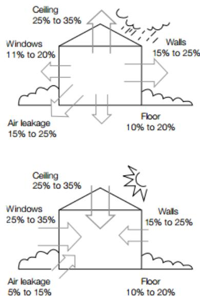
Figure 21 Typical Heat Gains and Losses in a Temperate Climate ([www.buildwise.org](http://www.buildwise.org))
