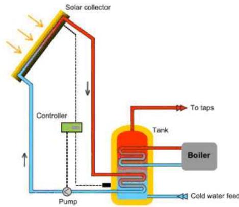
Figure 15 Solar thermal energy system for heating water (www.pres.org.pk).
