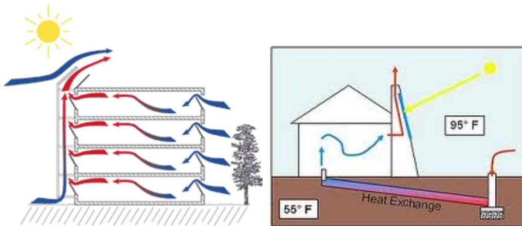
Figure 32 Solar Chimney ([passivesolar.weebly.com](http://passivesolar.weebly.com))
