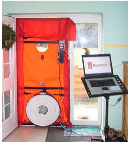
Figure 35 A blower door test measurement (energysolutionsnm.com)
