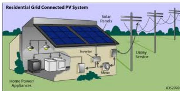
Figure 30 PV System ([www.infinitepower.org](http://www.infinitepower.org))
