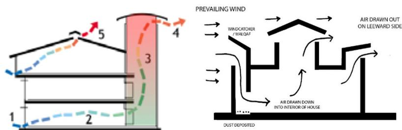
Figure 27 Solar chimney stack-induced cross ventilation (Inland Revenue Centre, ([www.cooneyarchitects.blogspot](http://www.cooneyarchitects.blogspot)))
