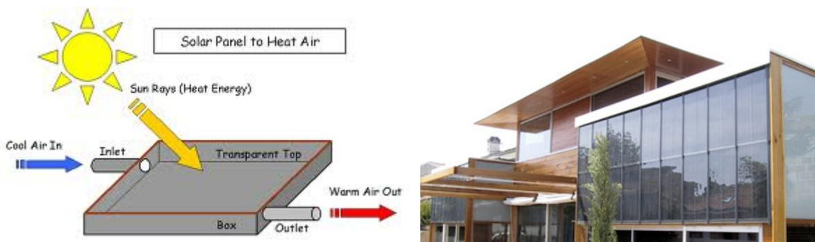
Figure 17 Solar thermal energy for heating air (www.makeitsolar.com)
