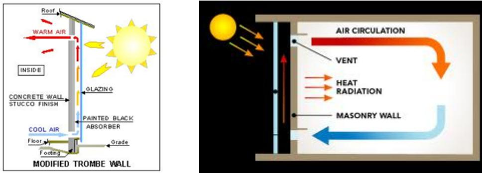
Figure 36 Working principle of Trombe Wall. (www.sierraclubgreenhome.com)
