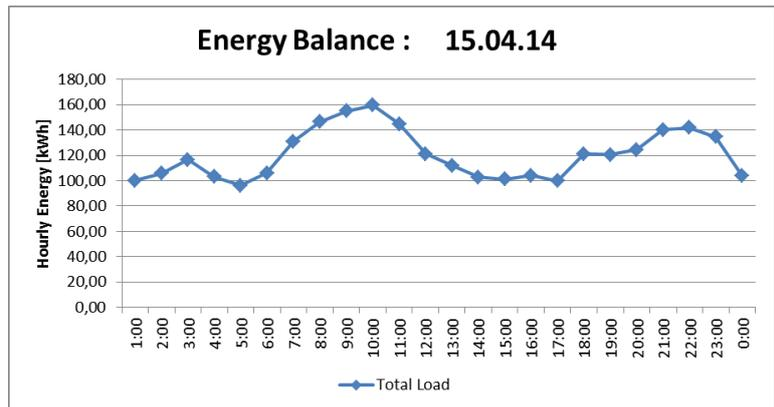
Figure 16: Total electrical load for the ORIGIN community Findhorn for one Tuesday in April 2014. The load profile shows consumption maxima in the morning and evening hours and a relatively high base load of nearly 100 kW. For more details please refer to the ORIGIN technical reports.
