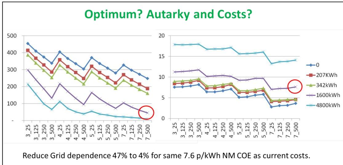
Figure 3: Left: y-axis = Grid imports (MWh per year), Right: y-axis = Cost in p/kWh of electricity supplied to the Community. x-axis = (#225kW wind turbines)\_ (kWp PV) (currently '3\_25' = 3 wind turbines, 25kWp PV). legend = kWh electrical storage. Red circles: 7 wind turbines + 500kWp PV + 1600kWh electrical storage gives only 50MWh per year grid imports and same p/kWh as current situation (currently 0 electrical storage).
