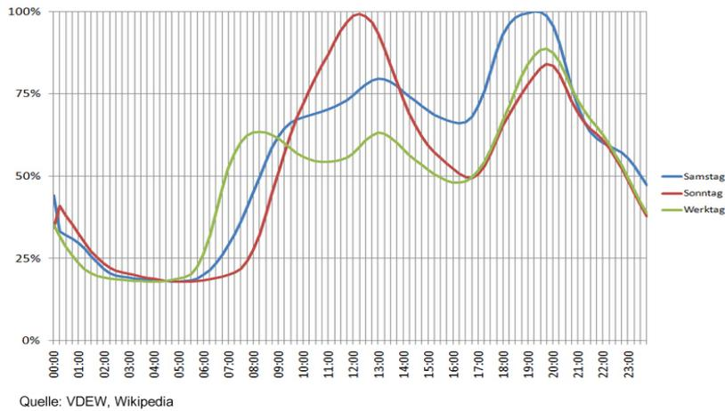
Figure 17: Standardised load profile H0 for household customers for different types of days during winter time. [Source: Wikipedia, based on data by German VDEW]
