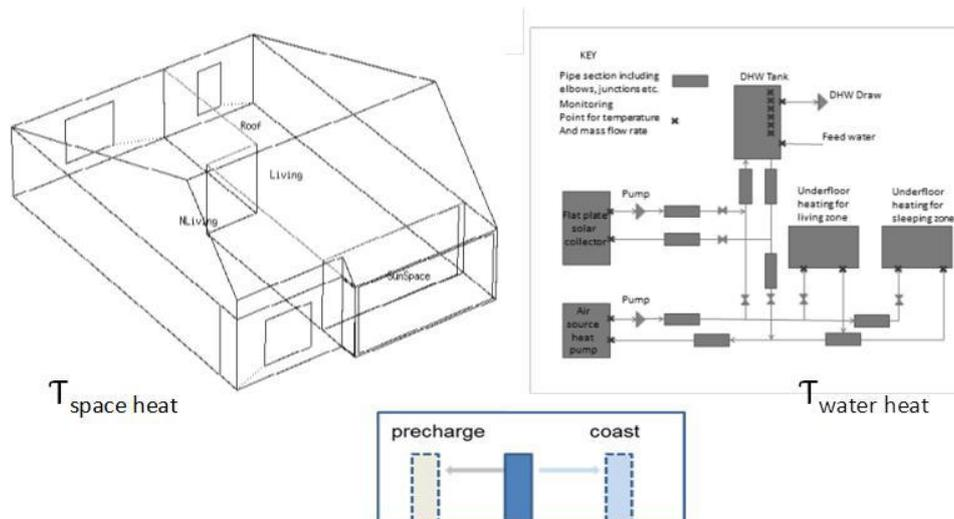
Figure 9: Detailed building and system models used to determine time constants for pre-charge and coast opportunity quantification for feeding into community level models (HOMER, MERIT) in the design stage.
