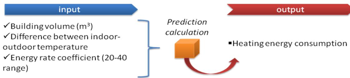
**Figure 17: Input and output for thermal energy prediction.**
