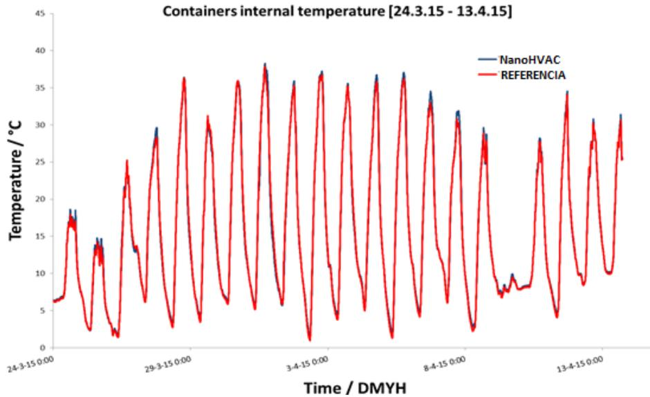
**Figure 3:** Thermal control of the demo buildings
