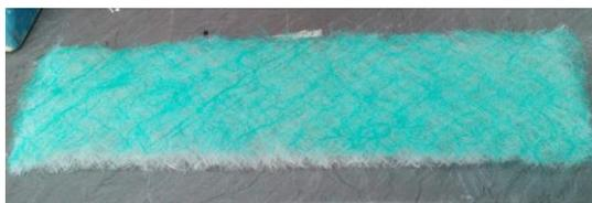
**Figure 6:** Filter covered by coating formulation developed by NANOPHOS
