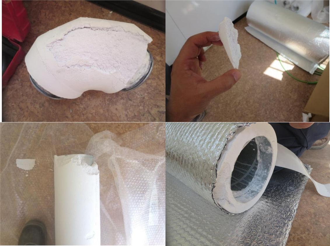
**Figure 13:** 40% of the NANOHVAC insulator was damaged. Poor mechanical properties
