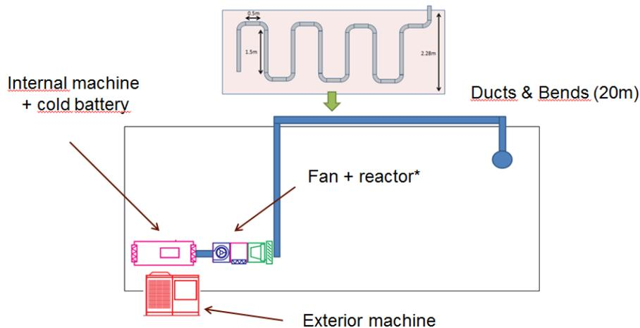
**Figure 12:** Scheme for installation of the NanoHVAC system
