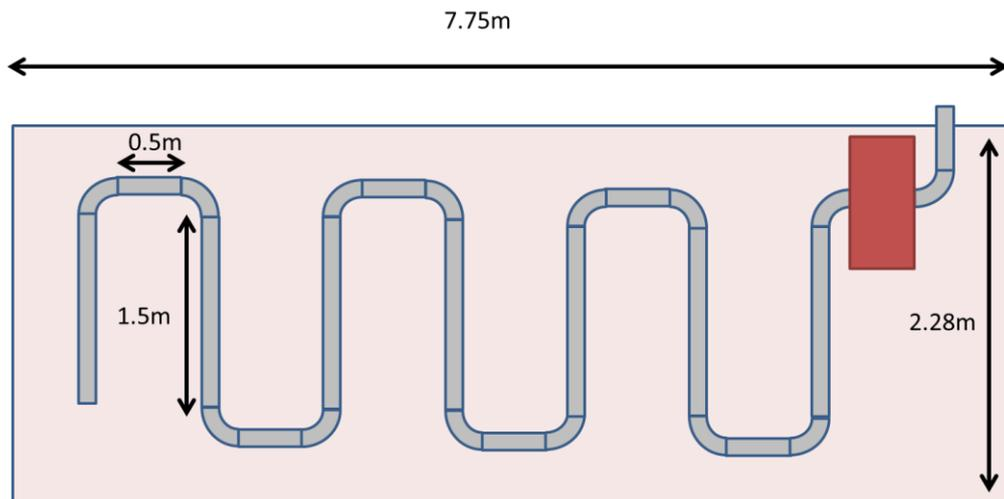
**Figure 4:** Geometry pipes for rooftop - "spaghetti form" for maximisation of bends
