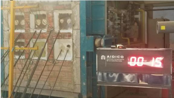
**Figure 24:** Panels at 15 min of test
