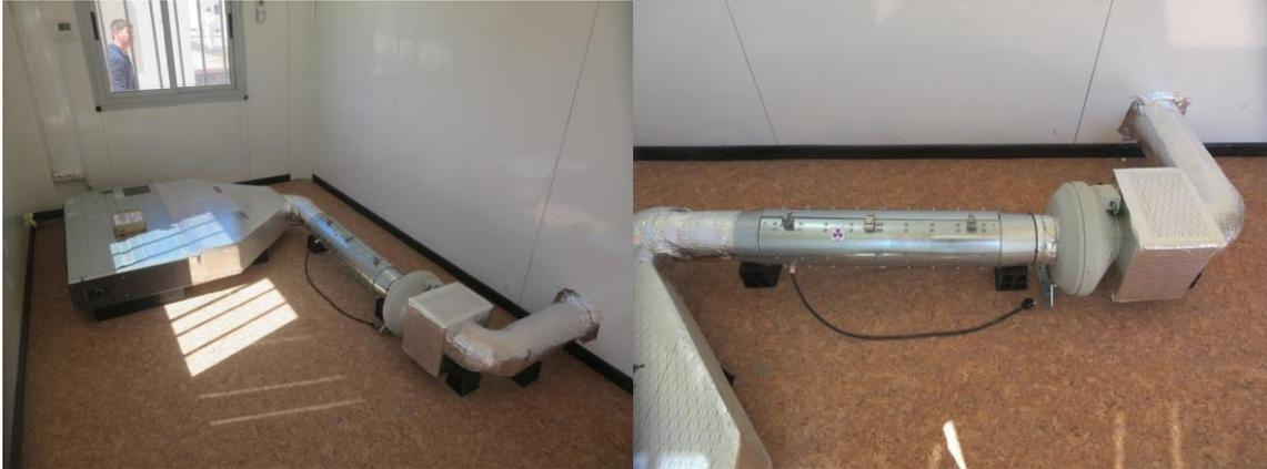
**Figure 17:** NanoHVAC interior machine + NTUA reactor + 180W fan
