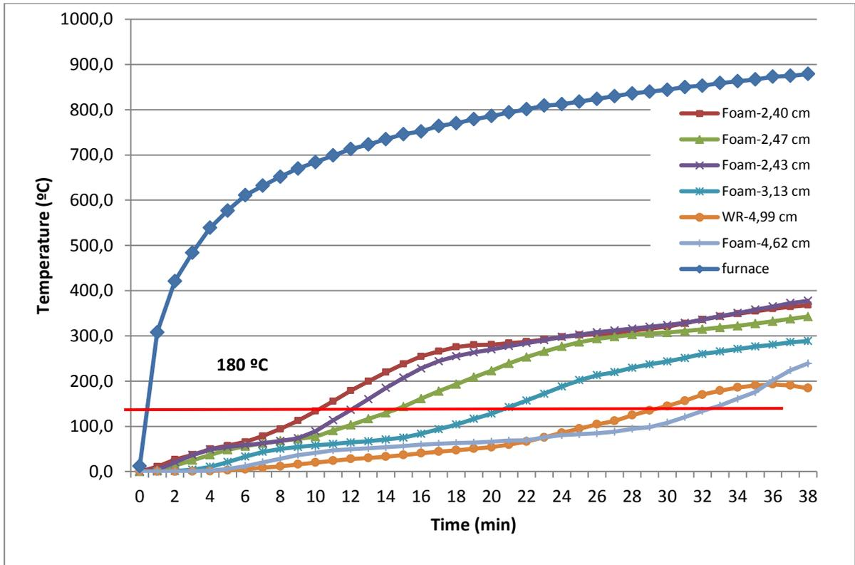
**Figure 28:** Temperatures curves of samples during the fire test
