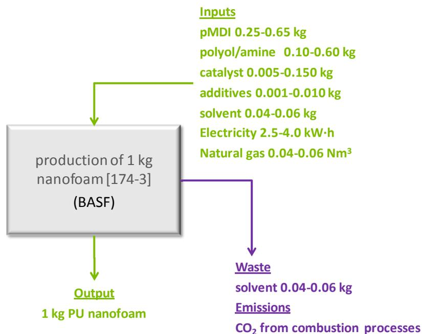
**Figure 7.** Input-output flowchart for production of 1 kg PU nanofoam.
