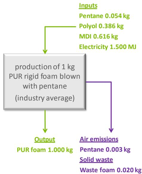
**Figure 3.** Input-output flowchart for production of 1 kg PUR rigid foam.
