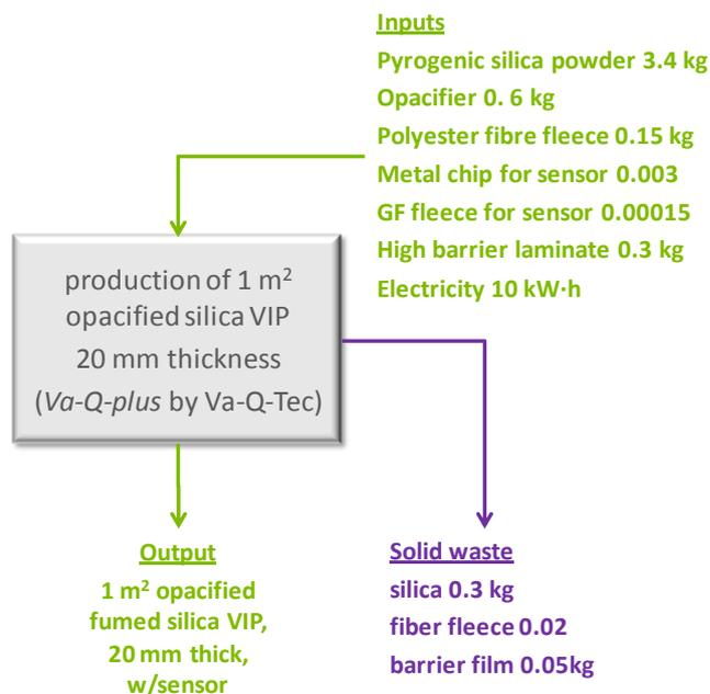
**Figure 4.** Input-output flowchart for production of 1 m<sup>2</sup> silica VIP.
