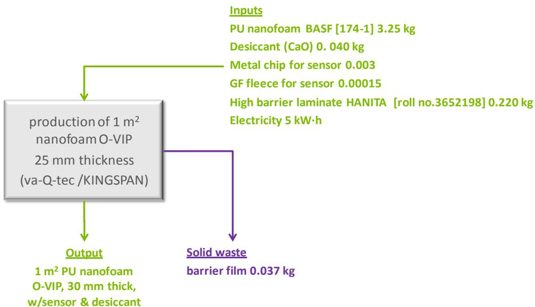
**Figure 6.** Input-output flowchart for production of 1 m<sup>2</sup> OVIP.
