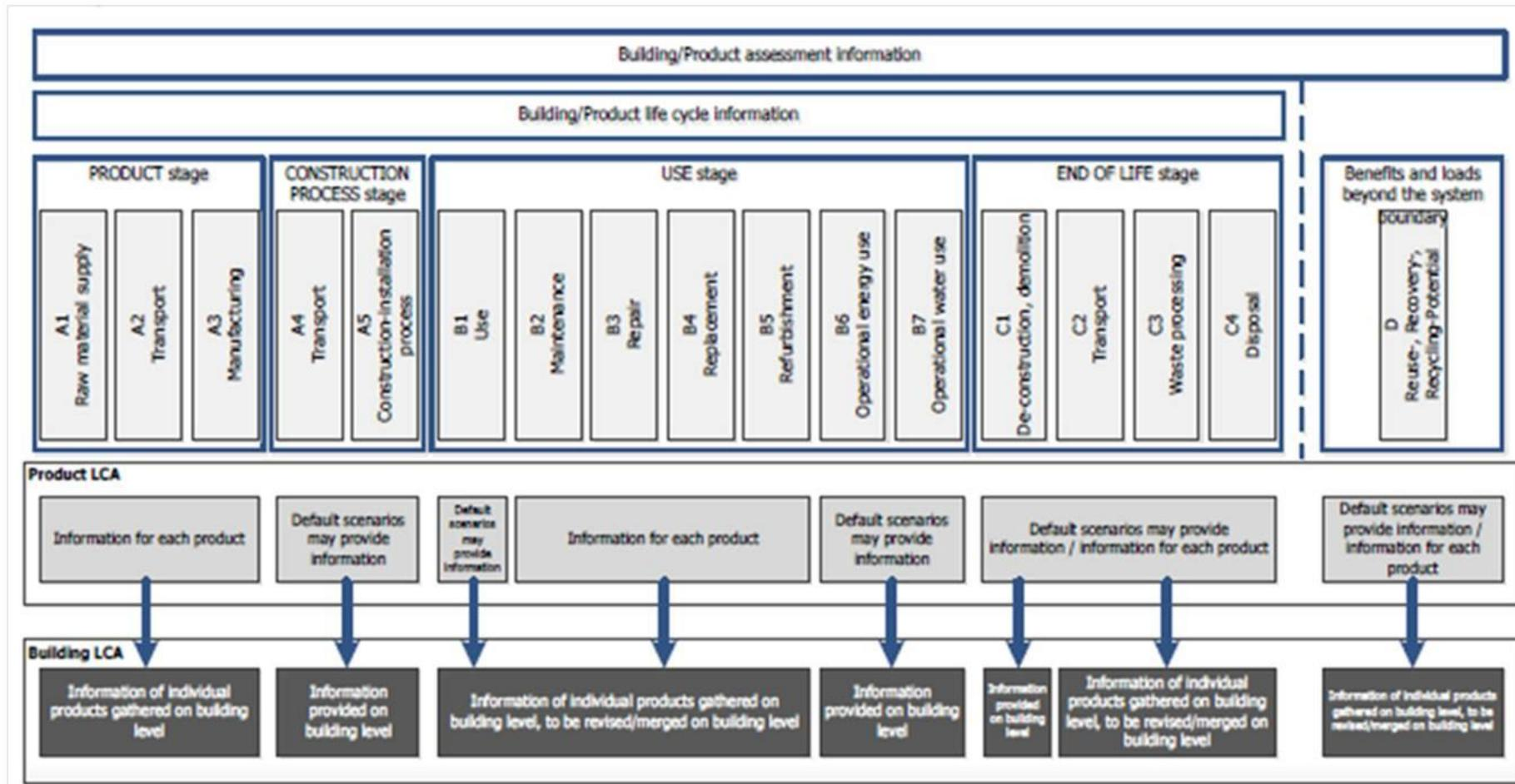
Figure 2. Modularity principle proposed by CEN TC 350 for the environmental evaluation in the EN standards.
