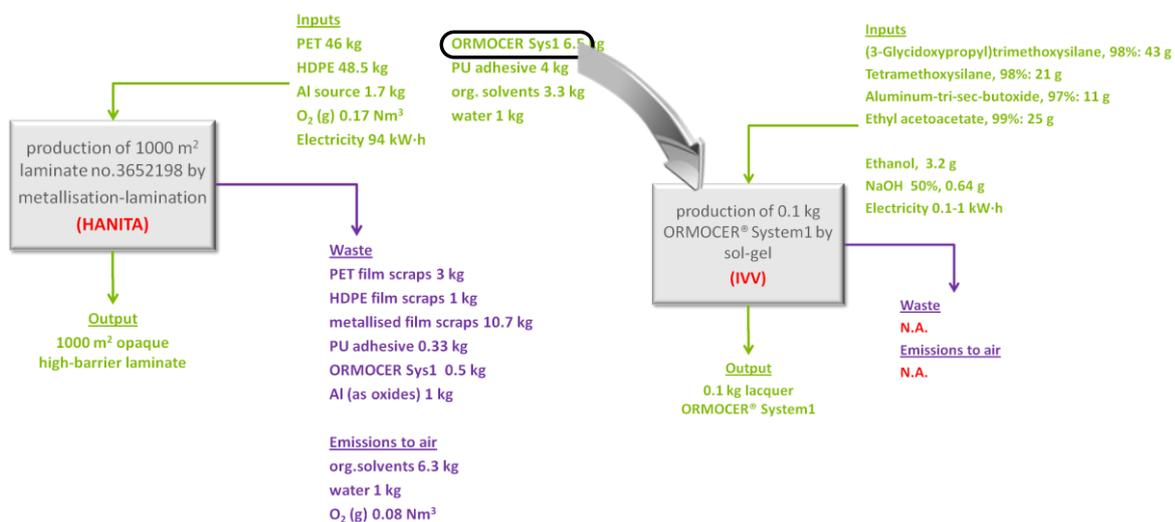
**Figure 8.** Input-output (aggreg.) flowchart for production of 1000 m<sup>2</sup> of advanced high-barrier laminate (opaque)
