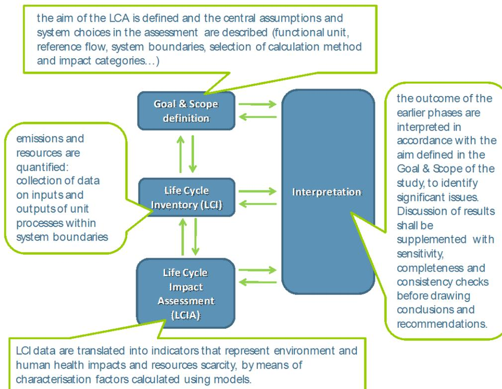
**Figure 1.** The four phases of a Life Cycle Assessment according to ISO 14040.
