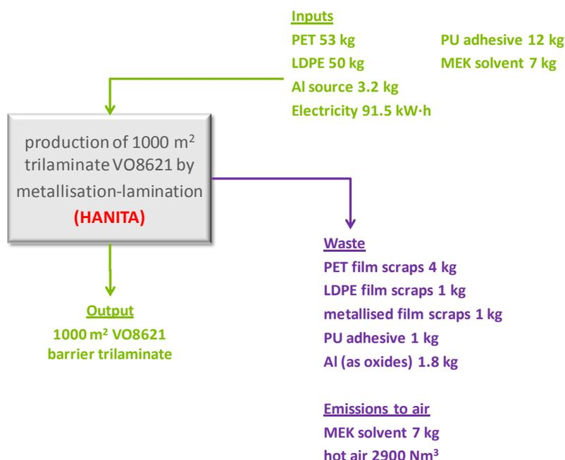
**Figure 5.** Aggregated input-output flowchart for production of 1000 m<sup>2</sup> VO8621 trilaminate film.
