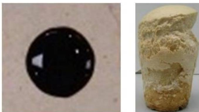
**Figure 63.** Single phase obtained as glycolysis product (left) and new foam formulated (right)
