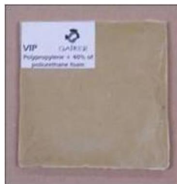
**Figure 59.** PP filled with PU foam from VIP waste (Source: GAIKER)
