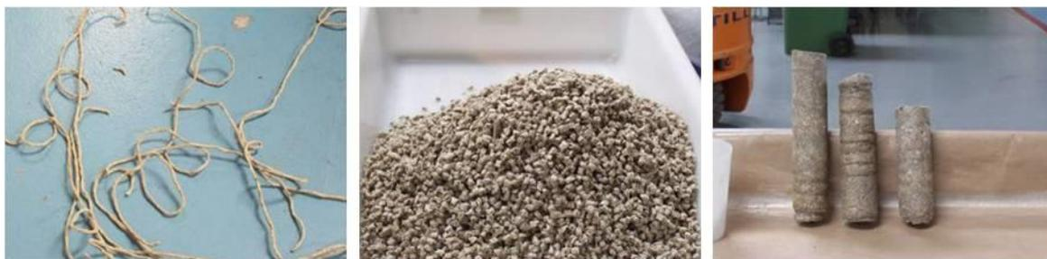
**Figure 68.** Extrusion products from multilayer films with aluminium (*Source: GAIKER*)
