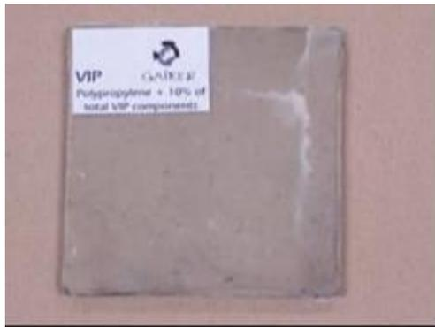
**Figure 40.** PP filled with silica VIP waste (Source: GAIKER)
