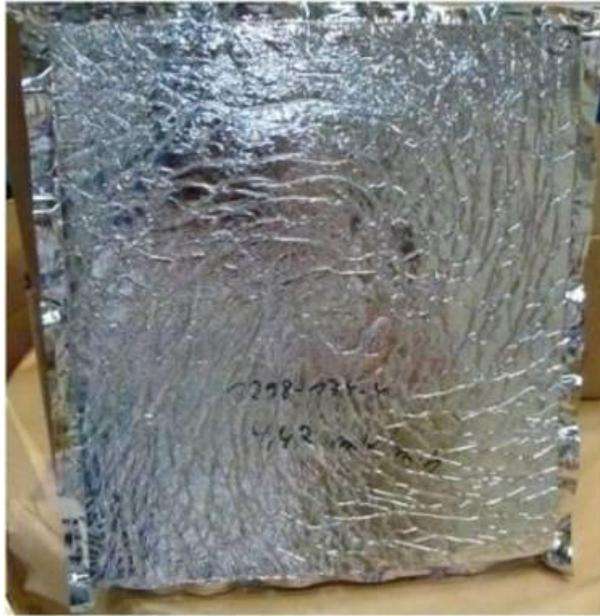
**Figure 18.** Sample of the O-VIP panel (BASF) received at GAIKER facilities.
