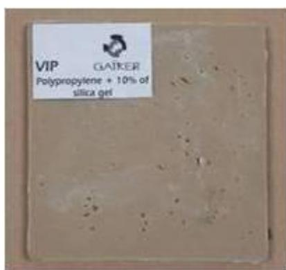
**Figure 55.** PP filled with fumed silica from VIP waste (Source: GAIKER)
