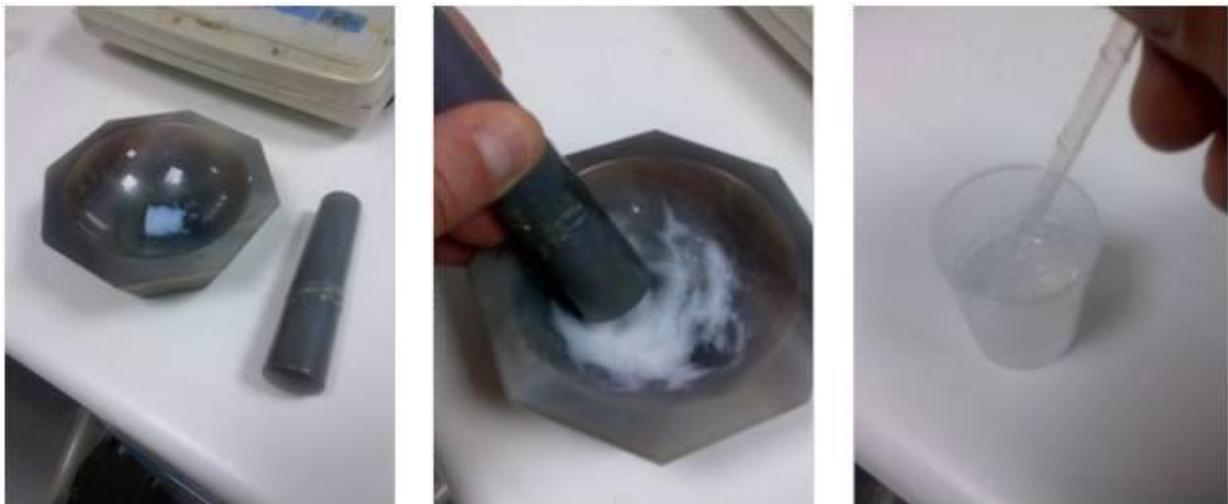
**Figure 49.** Sample preparation for viscosity measurement (first tests with aerogel sample coded ID 012 Pure TEOS)
