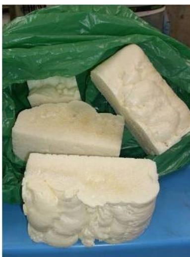
**Figure 62.** PU rigid foam used as feedstock for glycolysis evaluation
