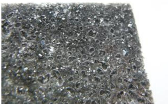
**Figure 66.** Porous back side of UP sheet filled with O-VIP film
