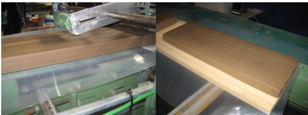
**Figure 8. Successful extrusion of 3I Binders**
