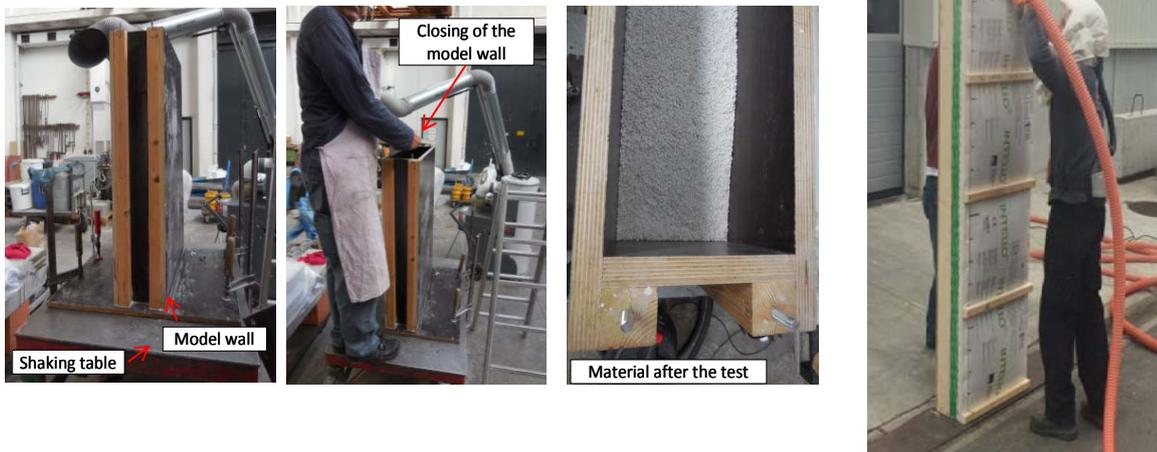
Figure 9. Application of 3I LFM for settlement testing
