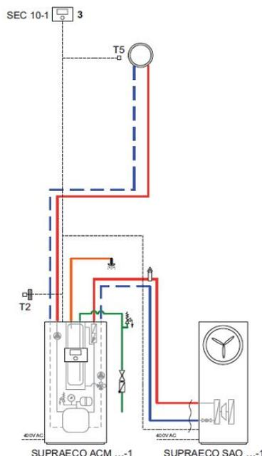
**Room temperature controller with 1 HC and integrated tank**
