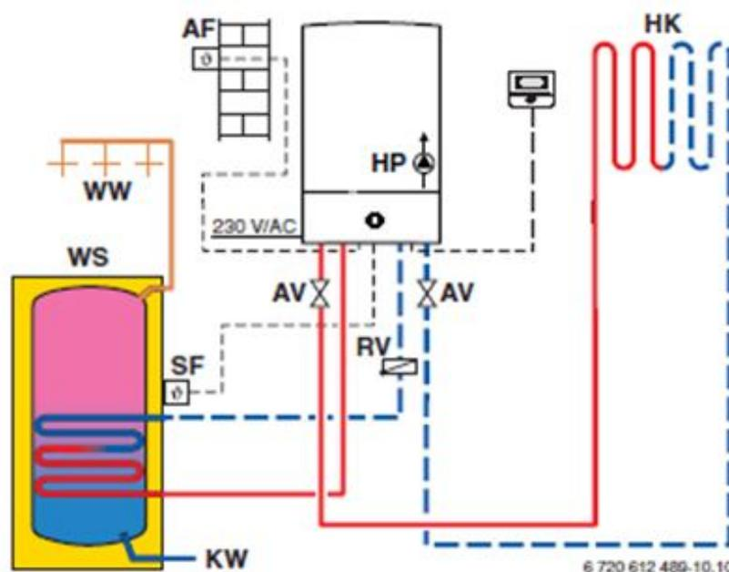
Weather depending controller with 1 HC and tank is often used with renewables. Generally condensing gas boilers are used with tanks and together with renewables (solar, solid fuel) in agrarian areas.
