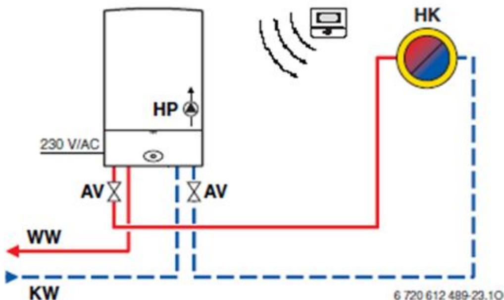
Room temperature controller RF with 1 HC and Combi boiler Generally condensing gas boilers are used (Combi boilers). Preferred controllers are room controllers (on/off) in RF-version
