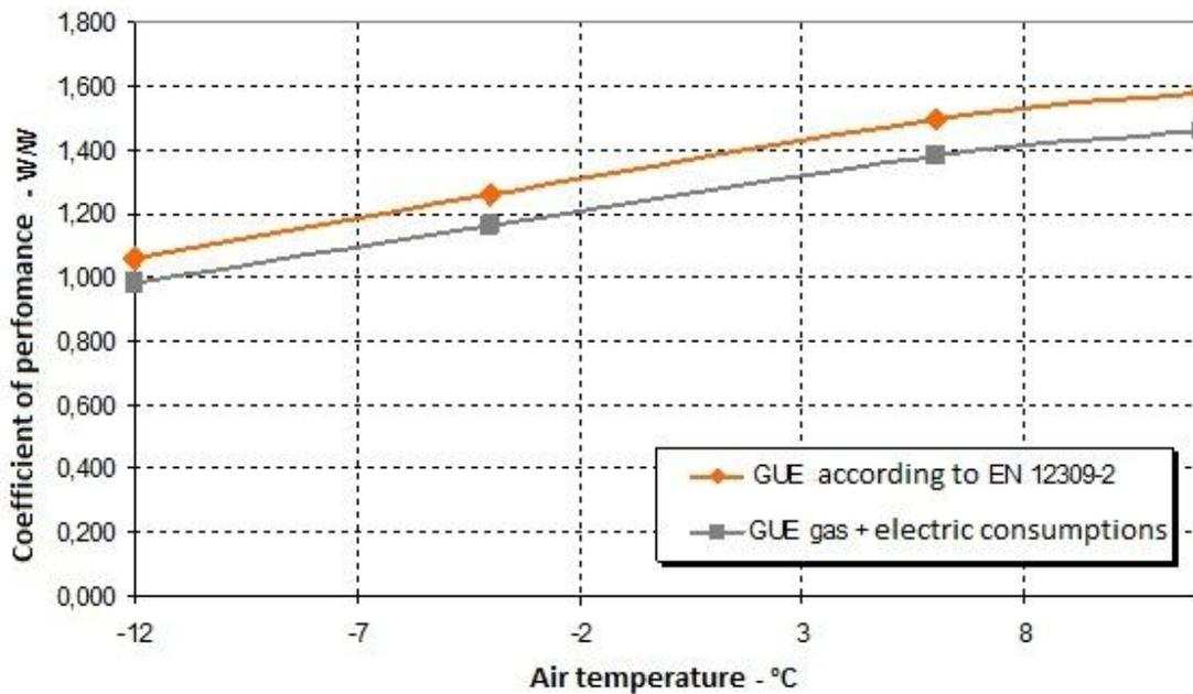
Thermal performance of an aerothermal GAHP (outlet 50° C)
