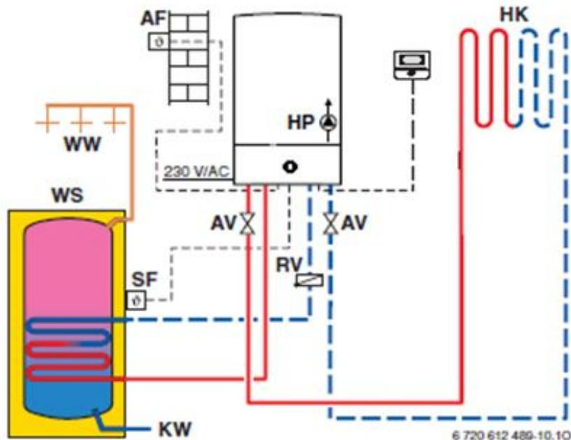
Weather depending controller with 1 HC and tank
