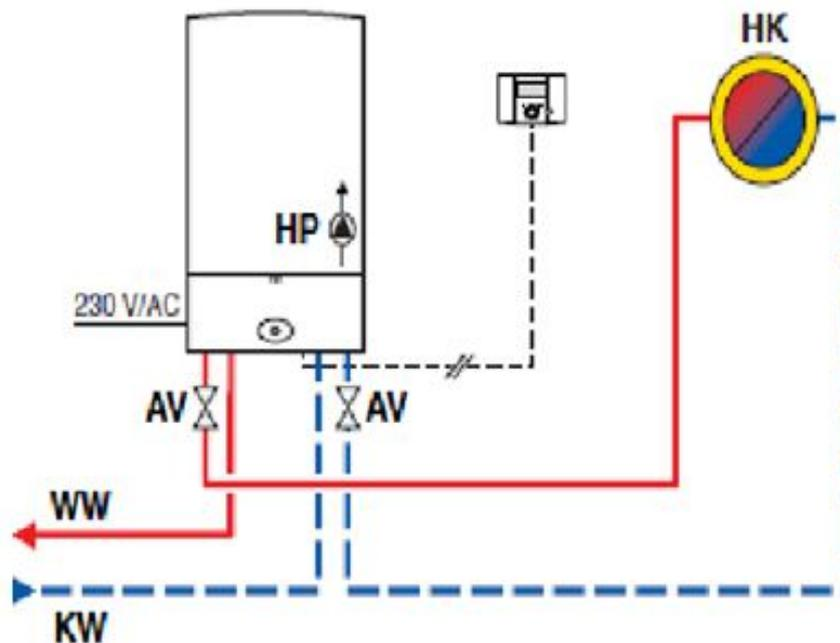
Room temperature controller with 1 HC and Combi boiler
