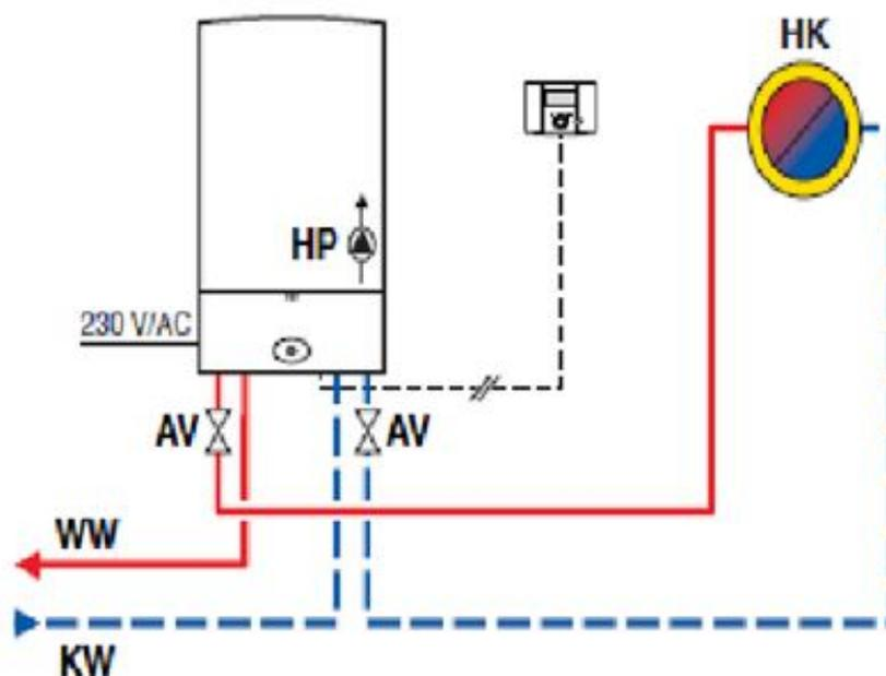
Room temperature controller OT with 1 HC and Combi boiler Generally condensing gas boilers are used(Combi boilers). Preferred controllers are room controllers (OpenTerm OT)
