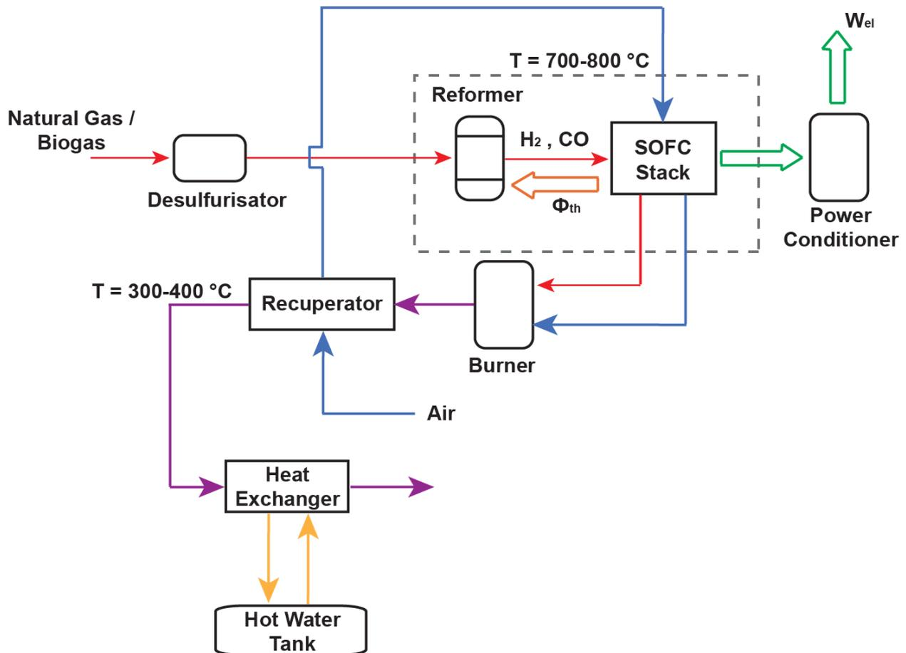
Figure C-2. Schematic representation of the FC-district  $\mu$ -CHP layout with steam-reforming fuel processor.
