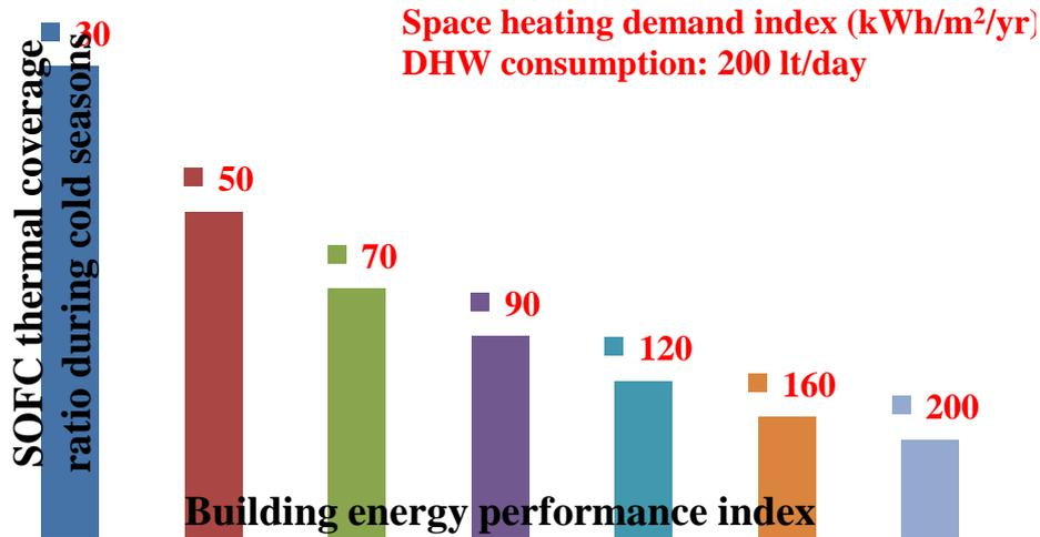
Figure A-3: Simulation of the share of the overall thermal demand provided by the SOFC to the ‘average’ household according to its energy performance index.
