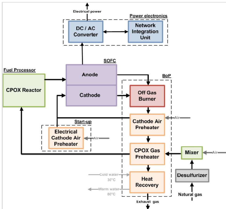
Figure C-1. Schematic representation of the FC-district  $\mu$ -CHP layout with C-POX fuel processor [7].
