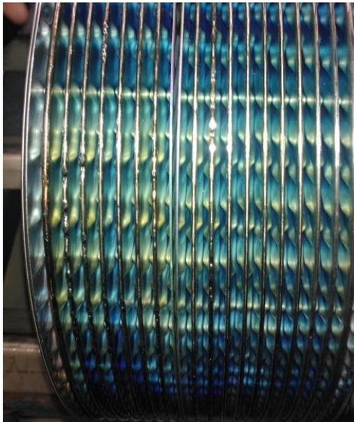
Figure 14: Coated plates welded at Vahterus
