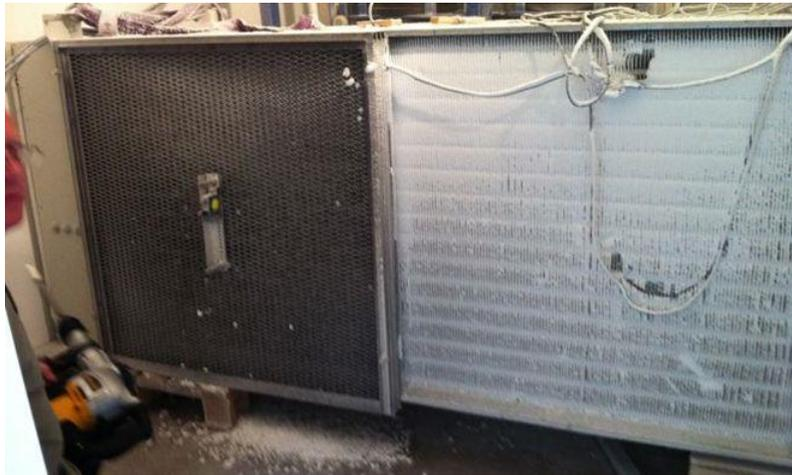
*Figure 2: Left side: Heat exchanger with meshes, frost free after vibration by a beat mill. Right side: Frost blocking an otherwise identical heat exchanger without meshes.*
