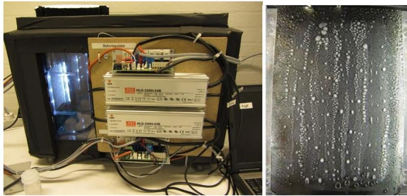
Figure 1: left: Freezing test chamber, on the left side, the sample plate (metallic blue) is mounted with a cooling block behind (not visible). right: Image from the camera mounted inside the test chamber. Frost on a bare Al-plate
