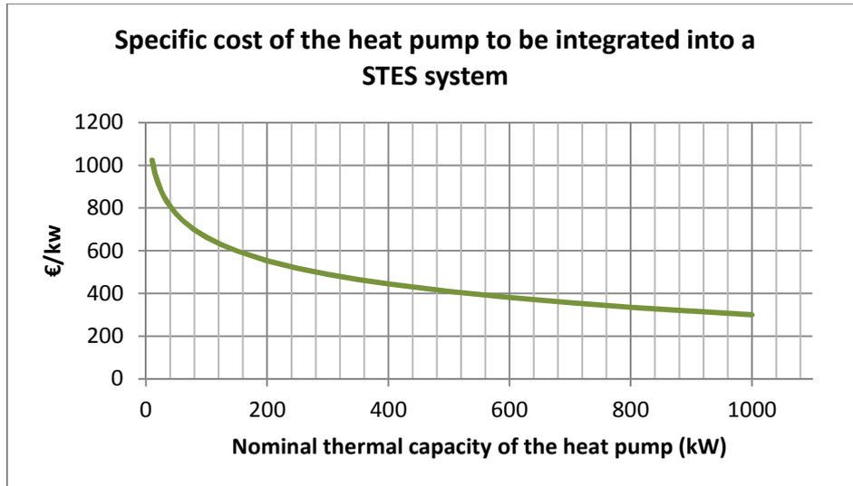
Figure 30: specific cost of the heat pump (source: Einstein project)
