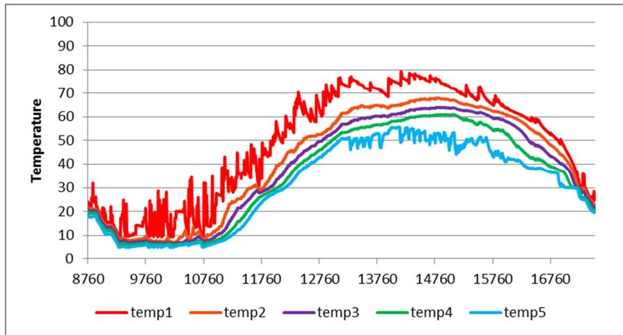
Figure 24: temperature profile inside the storage showing an inappropriate integration of the heat pump (too large)
