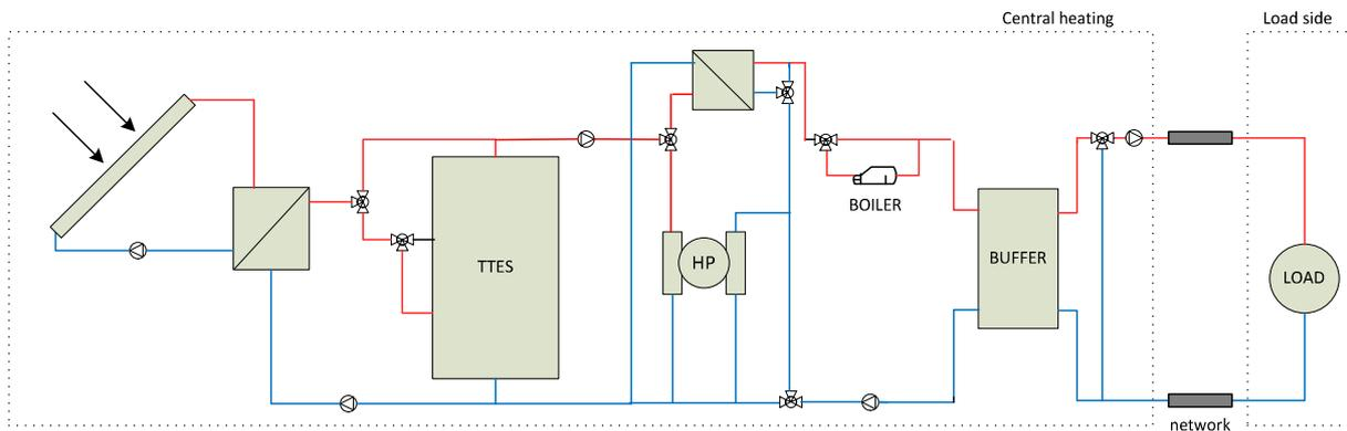
Figure 14: conceptual scheme for non-pressurized TTES with heat pump (source: Solites and Tecnia)
