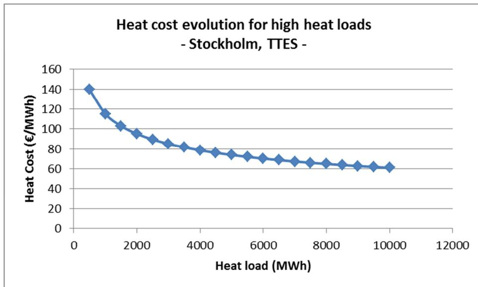
Figure 31: heat cost evolution against heat load for a STES system with hot water tank and a solar fraction around 60% for Stockholm
