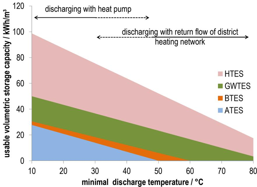
Figure 11: Usable volumetric storage capacity in dependency of the minimal discharge temperature of the different STES technologies depending on the return flow temperature of the district heating network and usage of heat pumps (source: University of Stuttgart)
