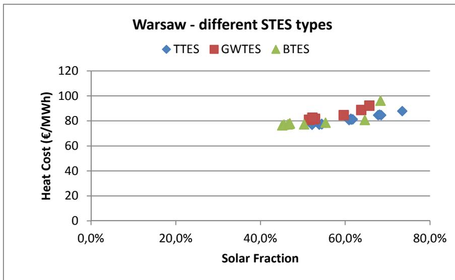
Figure 33: heat cost depending on the solar fraction for the considered case study in Warsaw. Boundary conditions of the simulations according to Annex 1.
