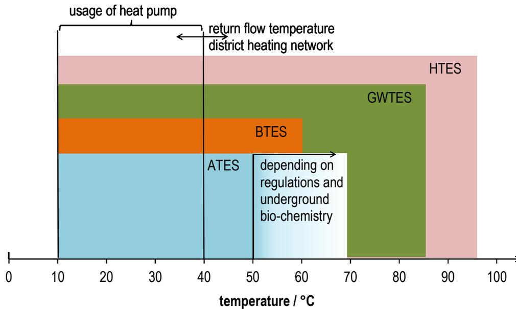
**Figure 10: Maximal operational temperatures of the different STES technologies depending on the return flow temperature of the district heating network and usage of heat pumps (source: University of Stuttgart)**
