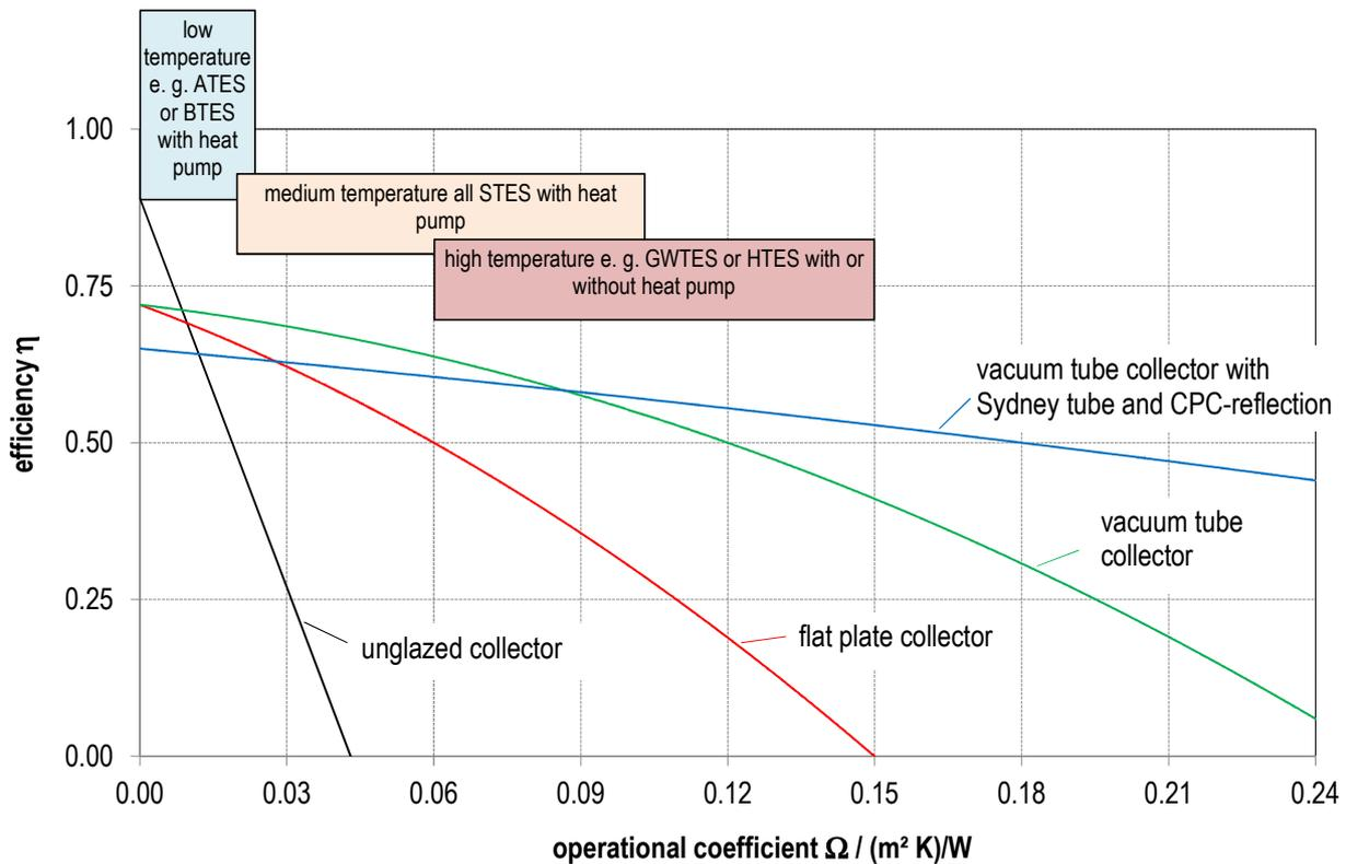
**Figure 9: Classification of solar thermal collectors for different STES and system integration by use of the collector efficiency and the operational coefficient, curves are based on aperture area (source: University of Stuttgart)**
