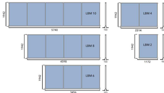
**Figure 6: Large-format flat plate collectors, LBM solution from Wagner Solar. Different sizes are available to ensure a customized solution**
