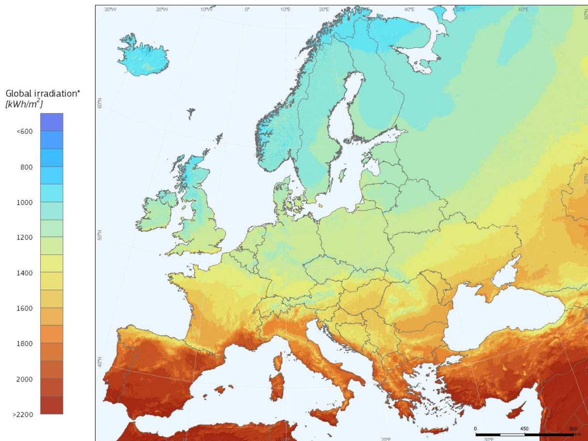
**Figure 1: Solar irradiation in Europe as annual sum (\*on optimally incident surface and azimuth directed to south) [5]**
