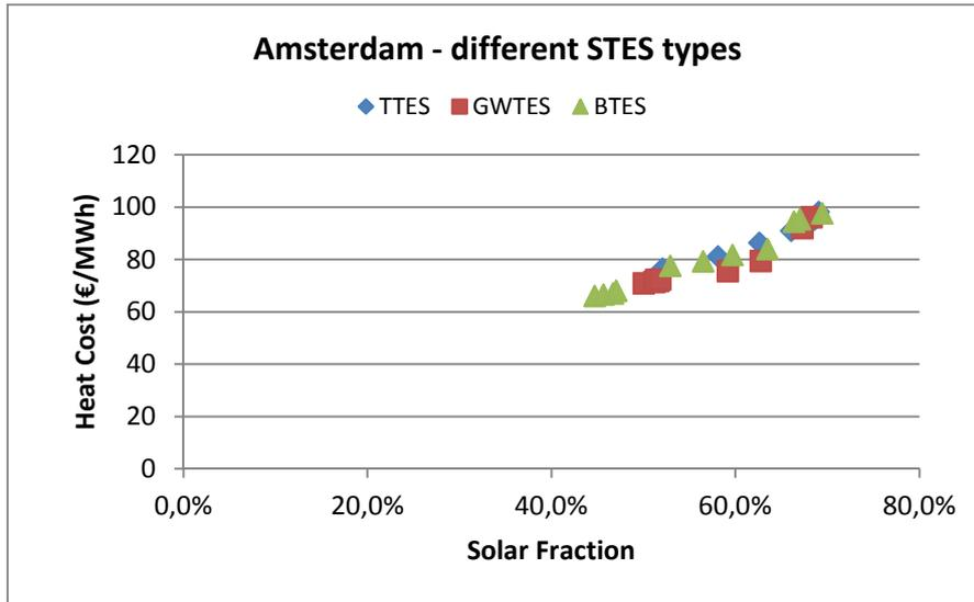
Figure 32: heat cost depending on the solar fraction for the considered case study in Amsterdam. Boundary conditions of the simulations according to Annex 1.
