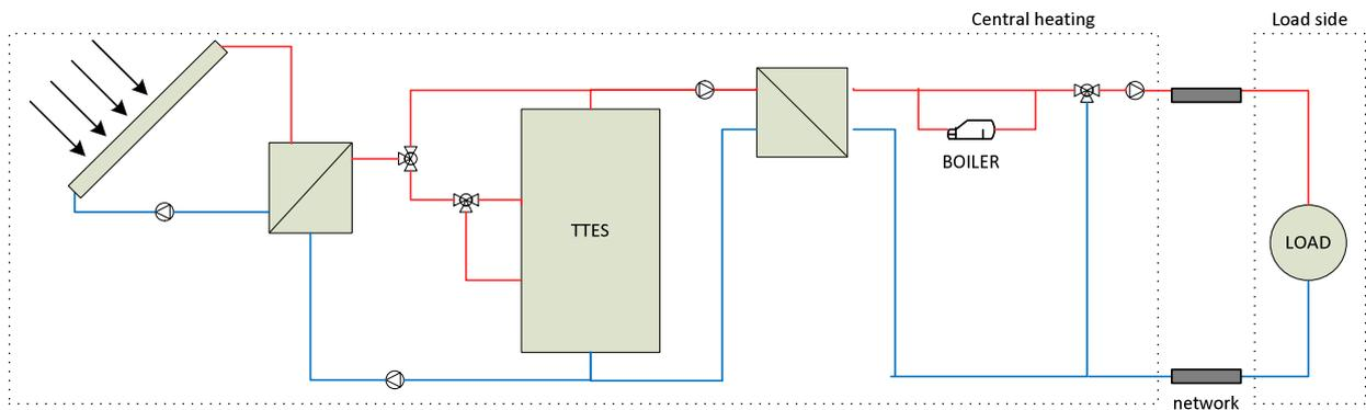
Figure 13: conceptual scheme for non-pressurized TTES without heat pump (source: Solites and Tecnalia)
