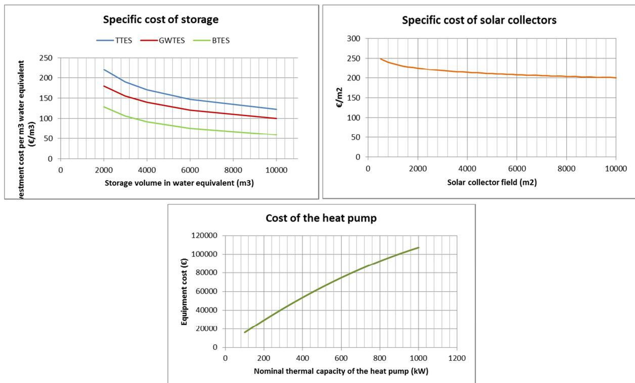
Figure 36: Specific cost of storage, specific cost of solar collectors and cost of the heat pump used for the simulations
