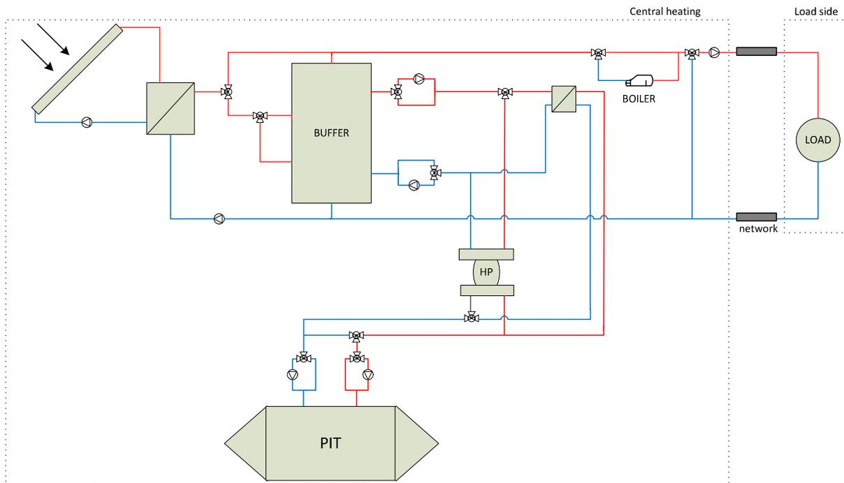
Figure 15: conceptual scheme for PIT with heat pump (source: Solites and Tecnalía)
