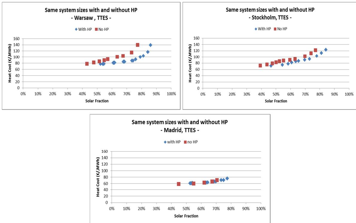
**Figure 21: Influence of the heat pump: simulation results of STES systems with and without heat pump. Heat pump capacity that best suit in each case: Amsterdam 650-800kW, Warsaw 650-800kW, Stockholm 400-800kW, Madrid 350-550kW.**
