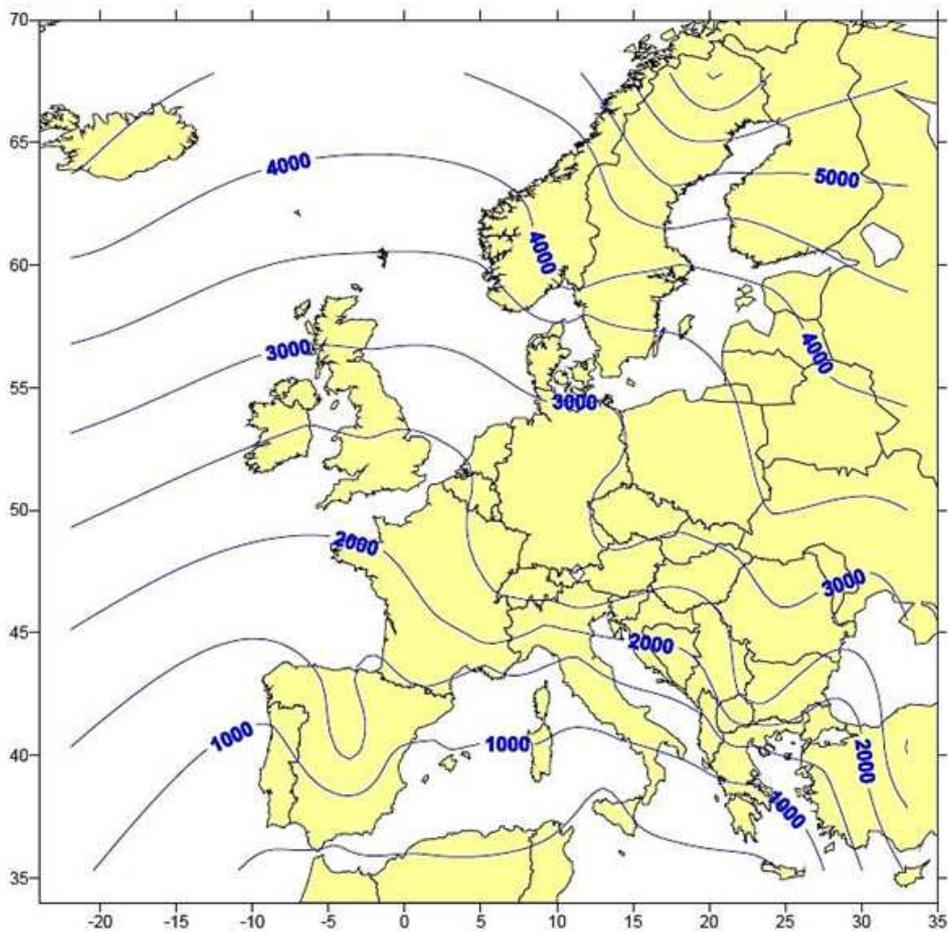
Figure 2: HDD isolines within Europe (source: Ecoheatcool and Euroheat & Power) [6]
