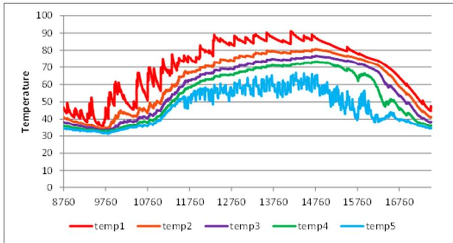
Figure 22: temperature profile inside the storage for a TTES without heat pump
