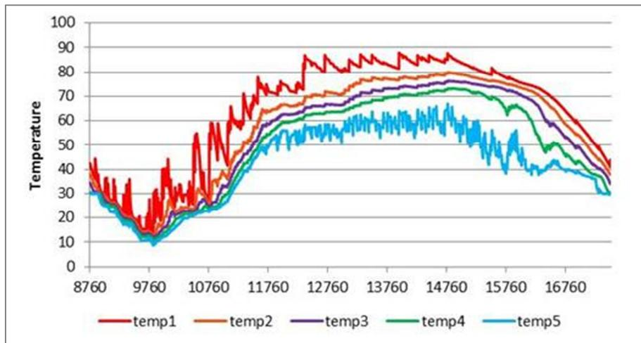
Figure 23: temperature profile inside the storage for a TTES with heat pump
