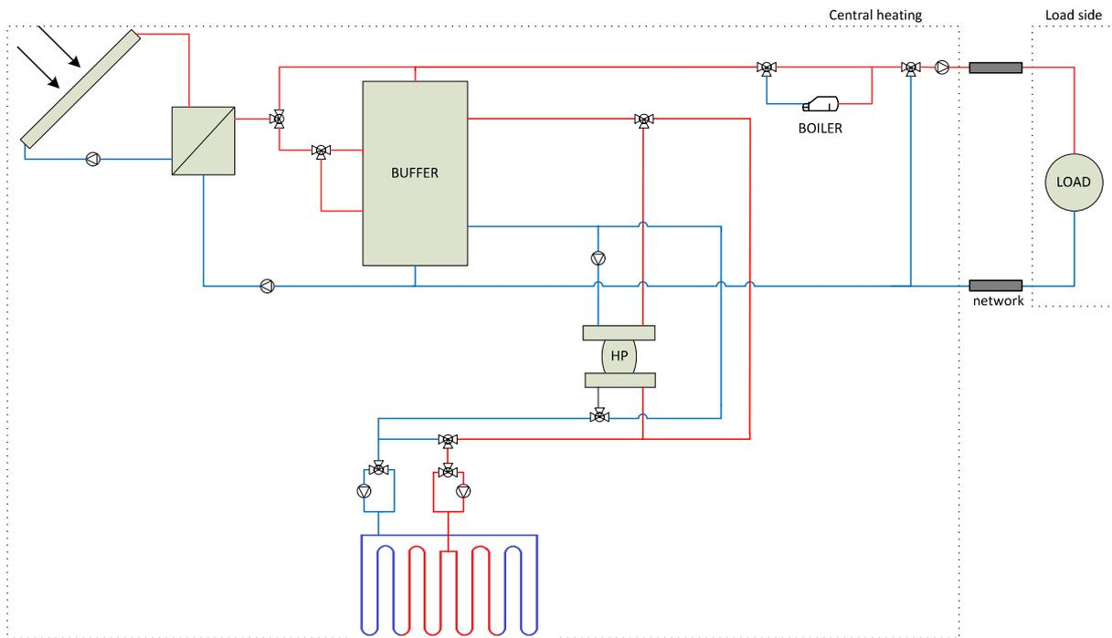
Figure 16: conceptual scheme for BTES with heat pump (source: Solites and Tecnalia)
