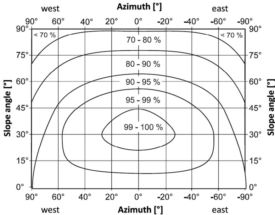
Figure 4: Potential annual solar irradiation in dependency of azimuth and slope angle as example for Germany [9]
