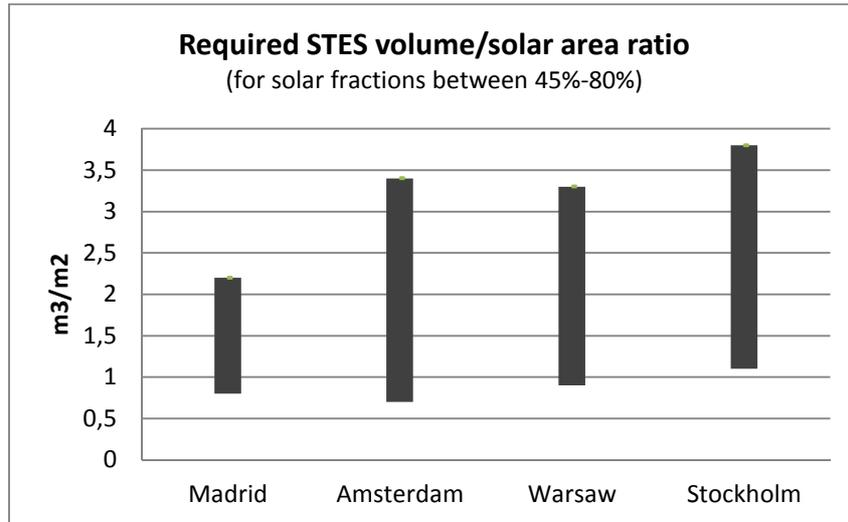
Figure 20: optimal storage volume / collector area ratio for Madrid, Amsterdam, Warsaw and Stockholm, for the boundary conditions and assumptions explained in Annex 1. The results include three STES types (TTES, GWTES and BTES); m<sup>3</sup> refers to water equivalent volume.
