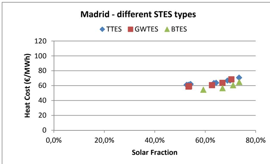
Figure 35: heat cost depending on the solar fraction for the considered case study in Madrid. Boundary conditions of the simulations according to Annex 1.
