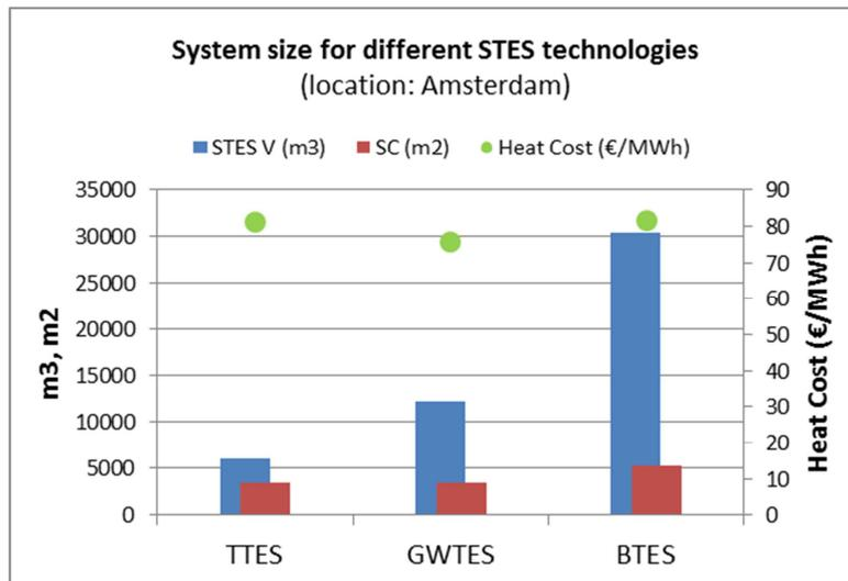
Figure 26: comparison of different STES types for a case study in Amsterdam, to achieve a solar fraction of 58% and primary energy savings of 38%.
