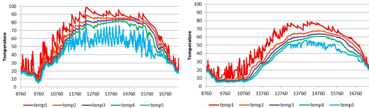
**Figure 19: temperature profile inside the STES for two different system sizes, representing situations with too small (left) and too large (right) storage volumes**
