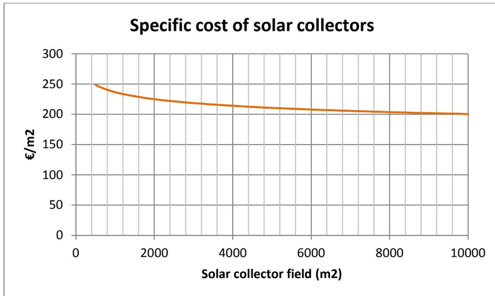
Figure 27: Specific cost of solar collectors. Source: Einstein project
