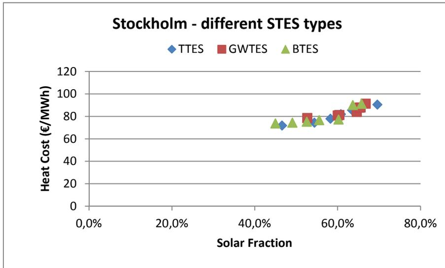
Figure 34: heat cost depending on the solar fraction for the considered case study in Stockholm. Boundary conditions of the simulations according to Annex 1.
