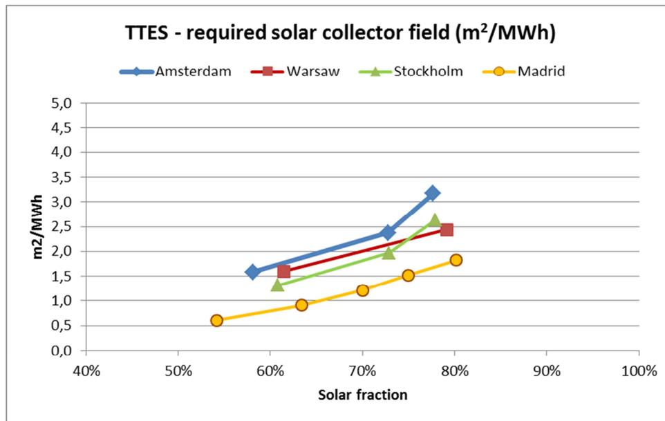
Figure 18: required solar collector area (m<sup>2</sup>/MWh) depending on the solar fraction for Amsterdam, Warsaw, Stockholm and Madrid. Considered STES type: TTES. Solar irradiance in the different locations: Amsterdam 1.129 kWh/(m<sup>2</sup>·a), Warsaw 1.106 kWh/(m<sup>2</sup>·a), Stockholm 1.204 kWh/(m<sup>2</sup>·a), Madrid 1.830 kWh/(m<sup>2</sup>·a).
