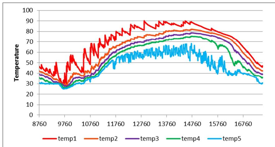
Figure 25: temperature profile inside the storage showing an inappropriate integration of a heat pump (too small)
