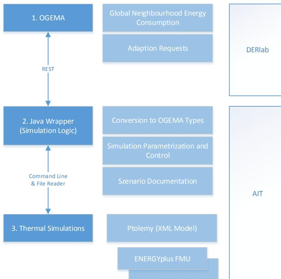
Figure 17. Operating Procedure between OGEMA and Simulation
