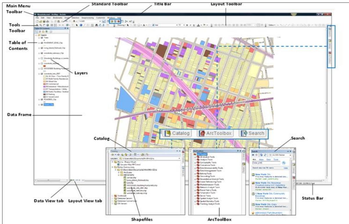
Figure 1. ArcMap as an example of a common GIS GUI
