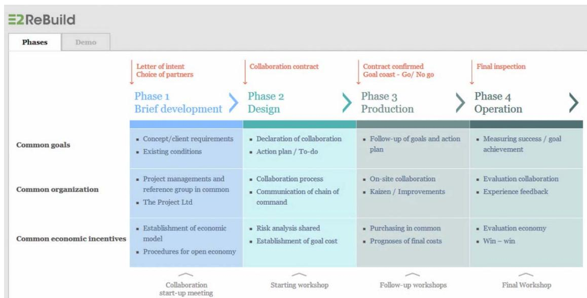
Figure 21: The four phases of the process map
