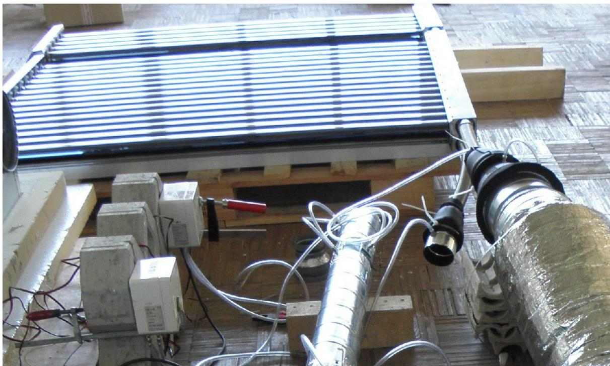
Picture 6: Kollektorfabrik test facility for pressure drop measurements of air collectors
