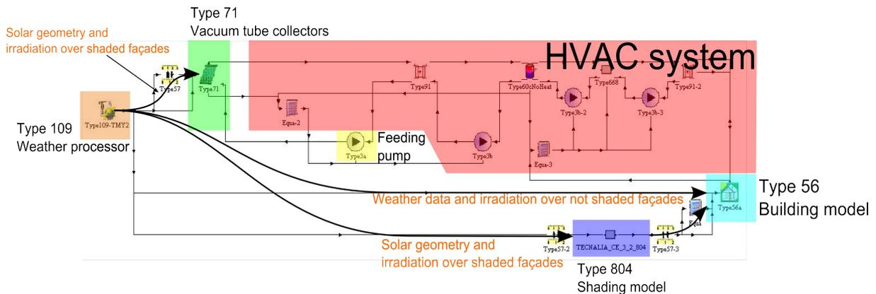
Picture 9: Model of a vacuum tube solar air collector for both HVAC and shading performance analysis
