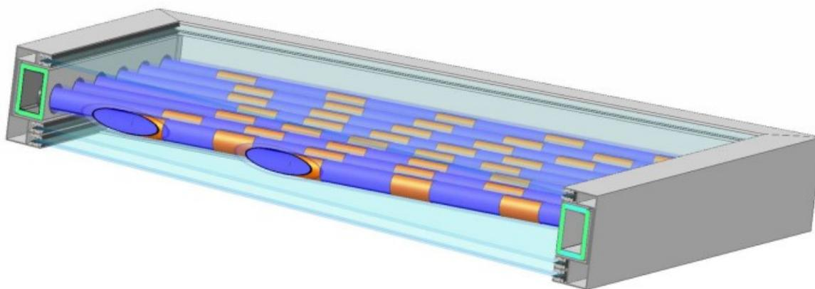
Picture 4: Sectional drawing of the new Cost-Effective air collector showing headers and continuous tubes
