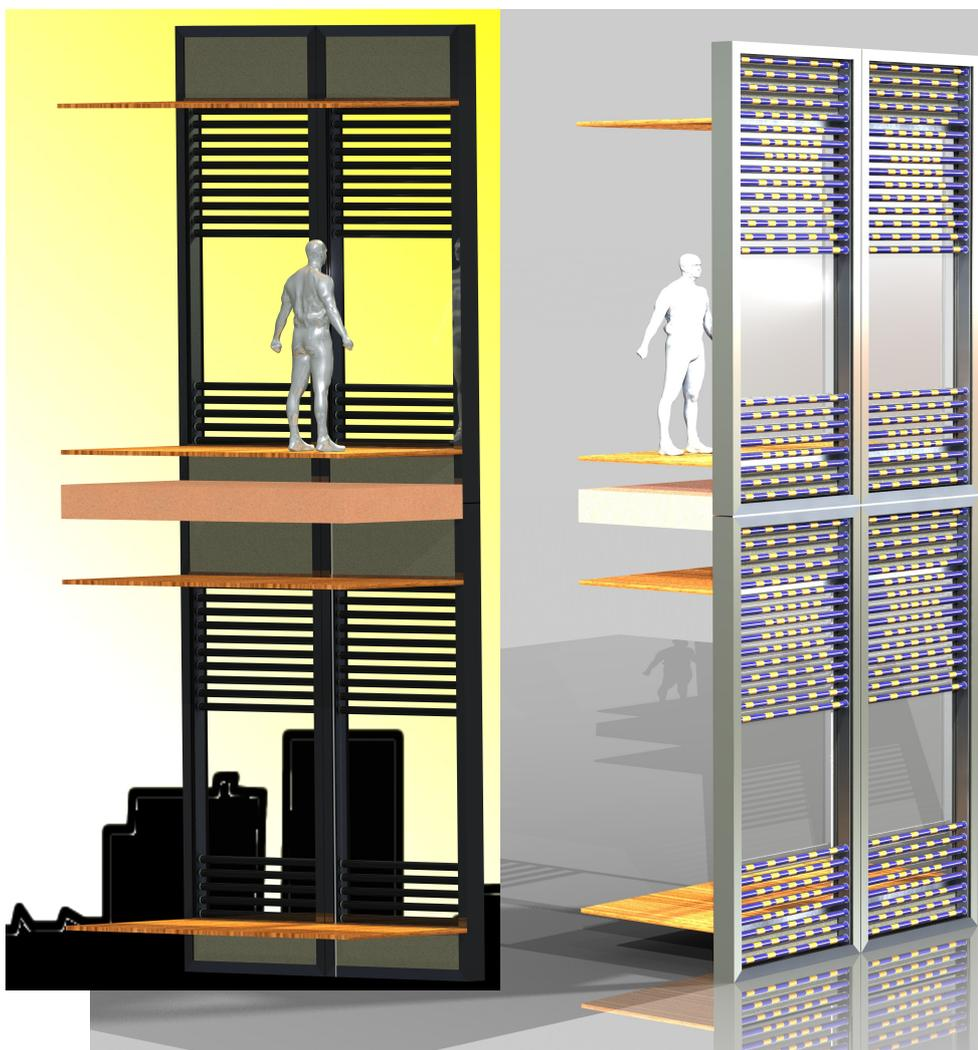
Picture 13: Drawing of a façade element with the new “Cost-Effective” vacuum tube solar air collectors.
