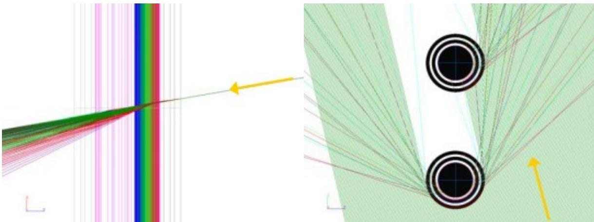
Picture 12: Simulating IAM - longitudinal (left) and transversal (right)
