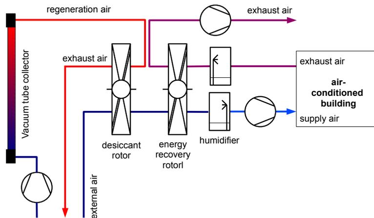
Picture 2: Example for a DEC cooling system driven by vacuum tube solar air collectors
