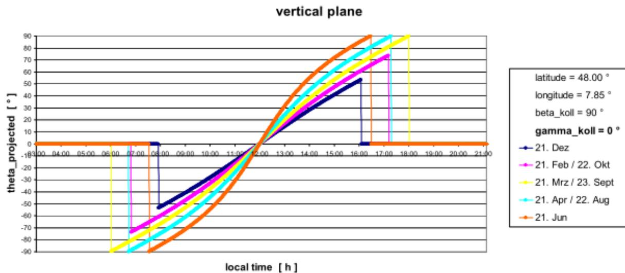
Picture 10: Incident angle of a vacuum tube solar air collector facing south
