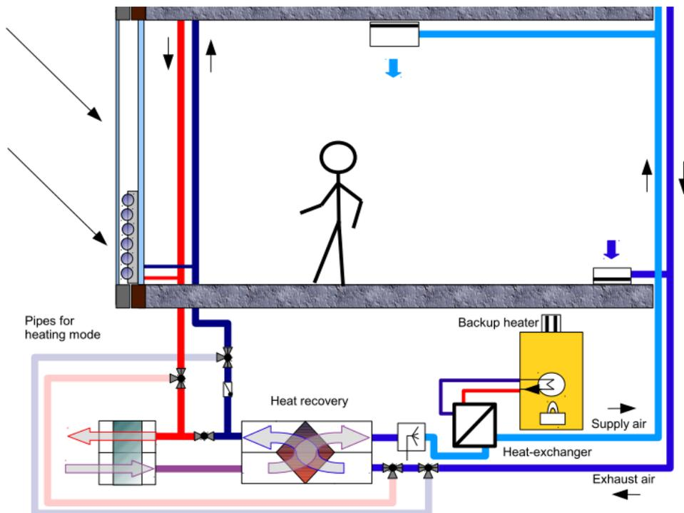
Picture 17: Example for cooling system with vacuum tube solar façade air collectors, Kollektorfabrik
