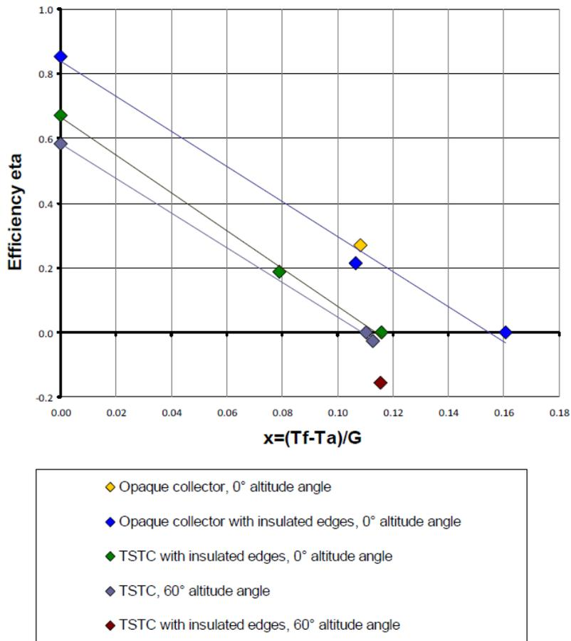
Figure 9. Collector efficiency curves.
