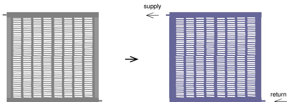
Figure 4. The absorber is first punched, then processed in a magnetron sputtering coater.
