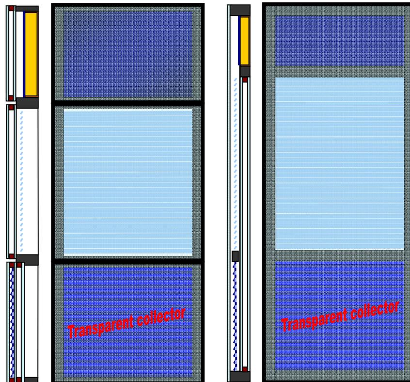
Figure 11. Collector may be integrated in the sill area of a single skin façade (left) or of a double skin façade (right).
