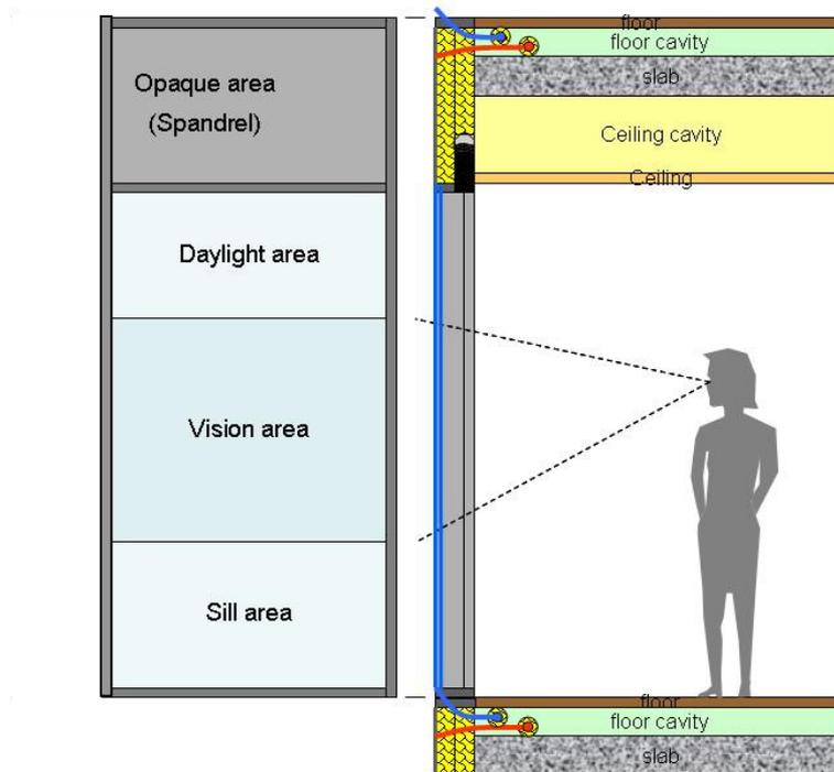
Figure 10. The different functional parts of the glazed area.
