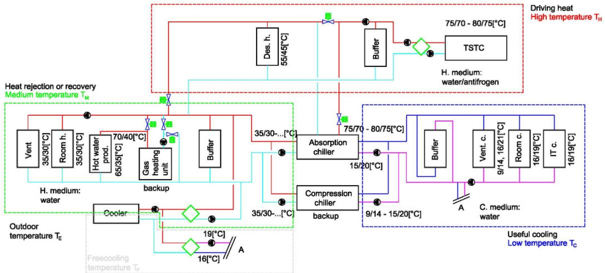
Figure 12. Scheme of the integration of the TSTC with the HVAC system.
