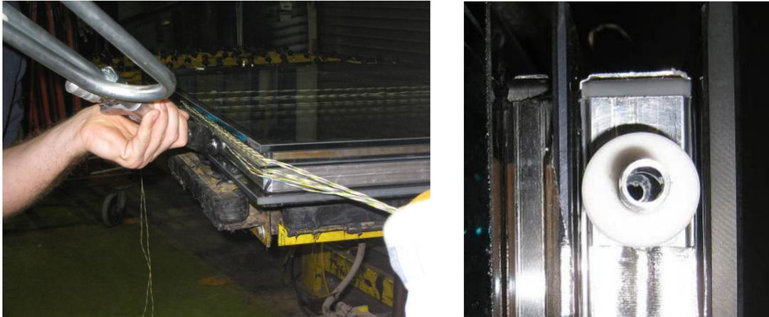
*Figure 6. Sealing of the triple glazing unit (left). The throughput connection (right).*
