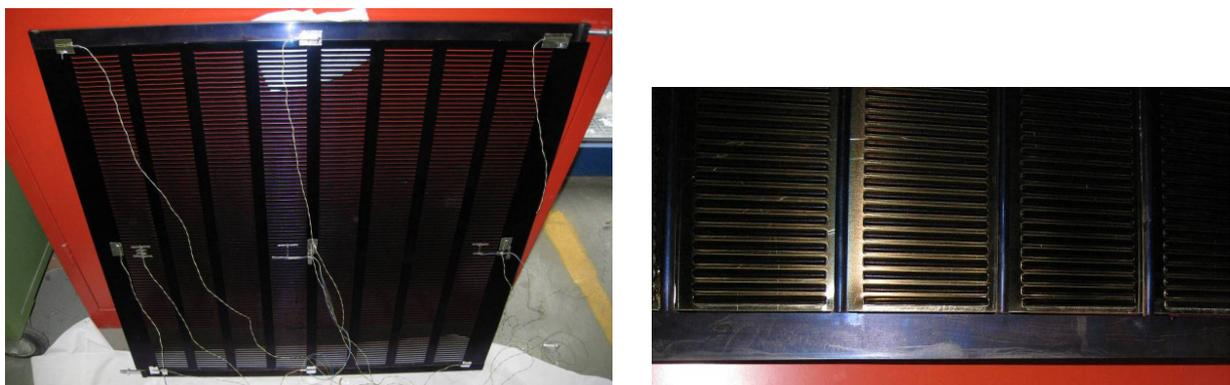
Figure 5. Finalized sample of the absorber and close-up picture.
