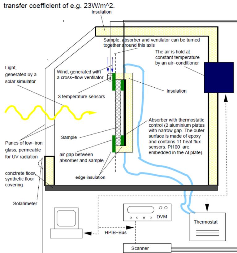
Figure 8. Cross section through the measurement chamber.
