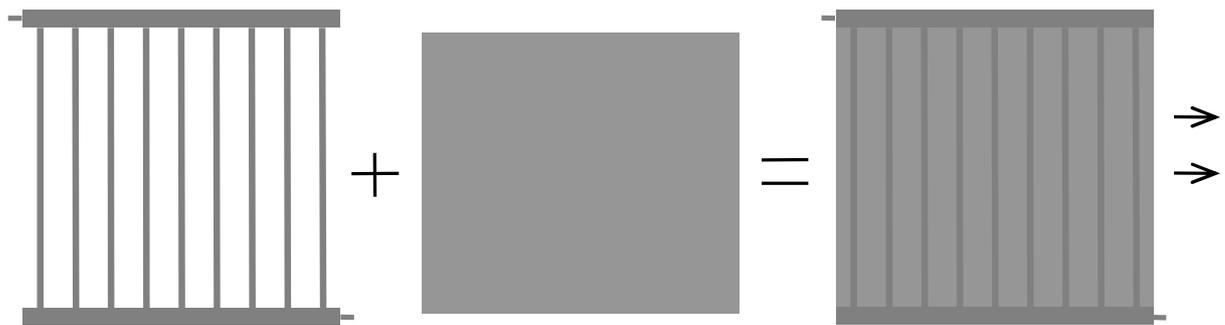
Figure 3. The aluminium pipe system is laser welded to a blank aluminium sheet to form a flat plate absorber.
