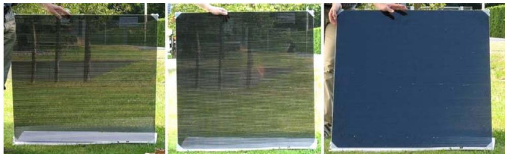
Figure 10: Photos of the first prototype. The angular dependency transmission is shown tilting the prototype from  $-30^\circ$  (very high transmission) to  $+30^\circ$  (the façade is more or less opaque).
