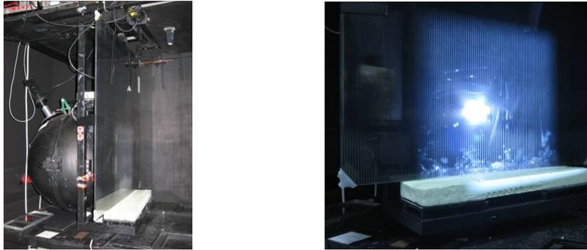
Figure 13: The images show the measurements in the Laboratory of Fraunhofer ISE. The first picture on the left represents the sample placed in front of the Ulbricht Sphere.
