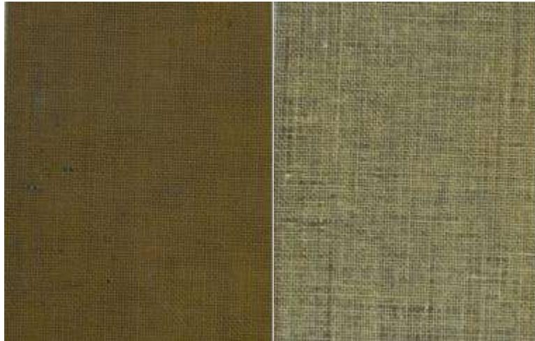
*Figure 3. Jute-biopolyester sample as moulded (left) and after 12w accelerated weathering (right) to illustrate the need for a weather resistant coating on the biocomposites.*
