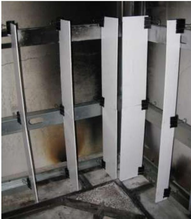
*Figure 13: Flax-Polyester small-scale ceiling lamellar prepared for fire testing.*
