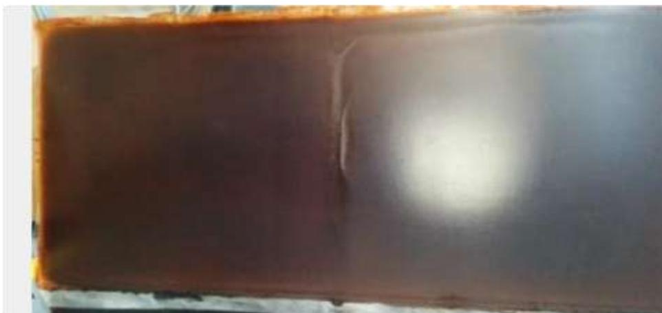
*Figure 10: A small-scale IPK skin made from fire retardant furan resin and jute.*
