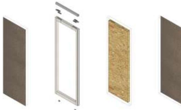
Figure 8: The BioBuild IPK panel planned construction components.
