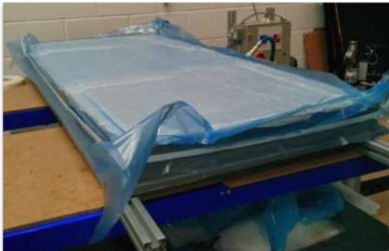
*Figure 9: Vacuum bagging process for production of small-scale IPK.*
