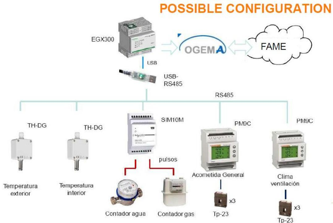
**Figure 20: draft architecture and commercial equipments to be installed in FCB stadium facilities**
